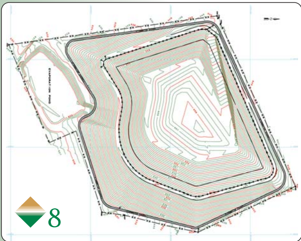
The phase 3 contour plan accommodates the final volumes of waste deposition and includes the eventual capping profiles required for efficient precipitation run-off after site closure.
